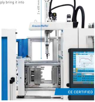
The telescoping stroke also permits use at low shop heights. The large remove stroke offers maximum flexibility.
