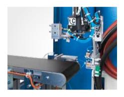
Compact conveyor belt integrated in the protective housing.
