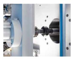
Flexible ejector coupling for fast setup, also available with adapter set
