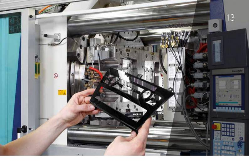
APC plus in the production of premium quality interior components with IML technology (Inmold Labeling) Sector: Automotive
